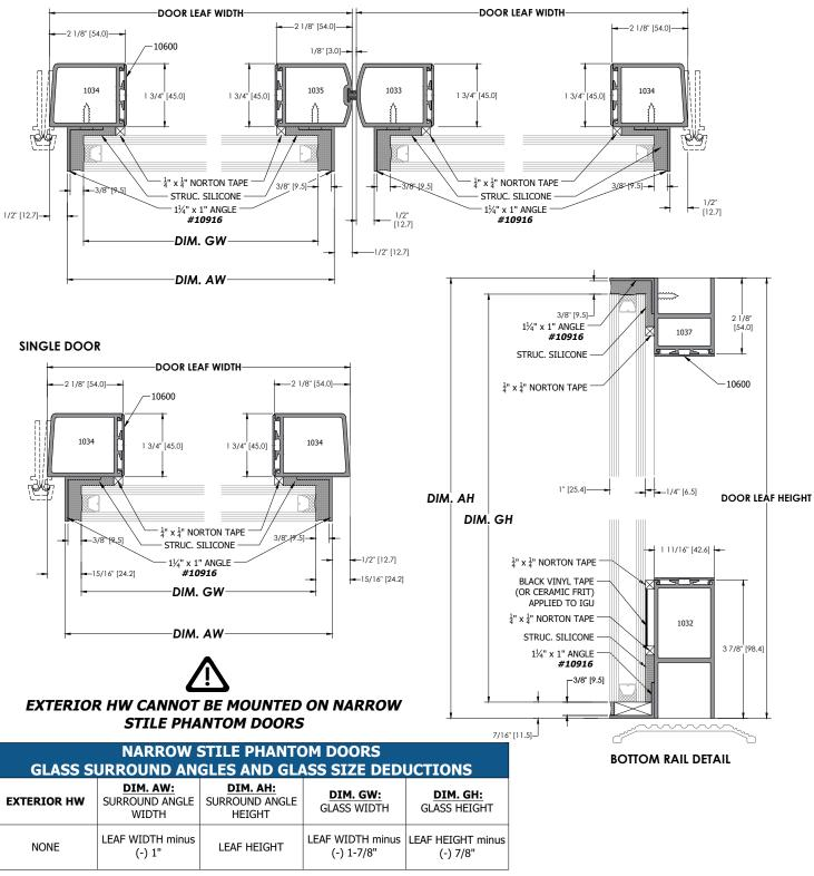
IGUS, VINYL TAPE (OR CERAMIC FRIT) ON IGUS, AND NORTON TAPE ARE NOT SUPPLIED BY ALUMICOR. Phantom Door Glazing Instructions
